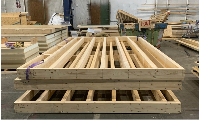
Figure 10.6 Timber frames, stacked in the factory, before the insulation and sheathing boards are applied.
