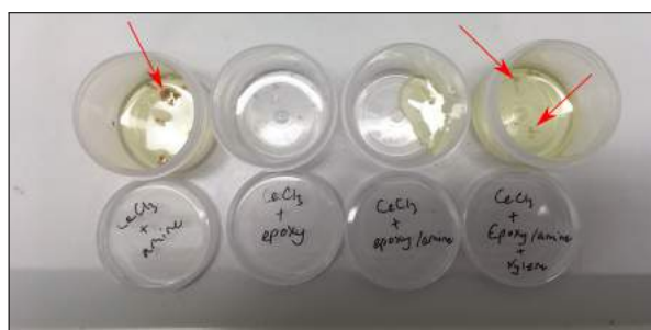
Figure 5.4: Reactivity between cerium and different coating components. From left to right Ancamine 2500, Epikote 828, Ancamine/Epikote mixture, Ancamine/Epikote/xylene mixture with some added \text{CeCl}_3 crystals. In the presence of amine-groups the cerium turns brown. Pure amine reacts faster and shows a more intense colour change compared to a mixture of Epikote and Ancamine. When xylene is added, the reaction takes place at a faster rate.
