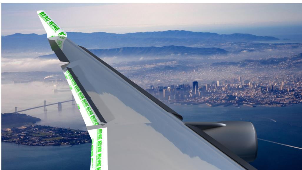
Figure 4.2: The Airbus A330 retrofitted wing with a 0° cant extended wingtip.
