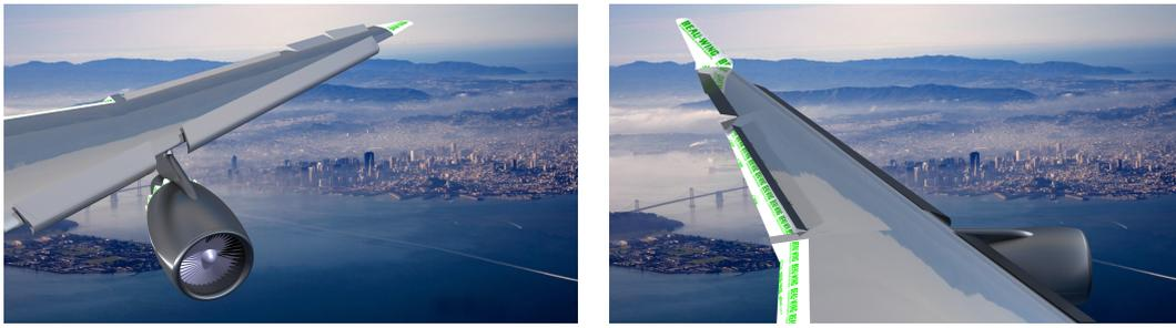
(a) The Airbus A330 retrofitted wing with a 90 degrees cant extended wingtip.
