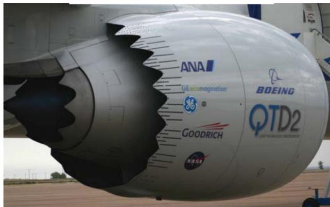
Figure 3.3: AVC installed on the Quiet Technology Demonstrator 2 airplane by Boeing [9].
