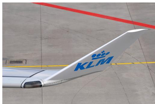
Figure 3.24: The winglet of an A330, with the lighting system clearly visible.
