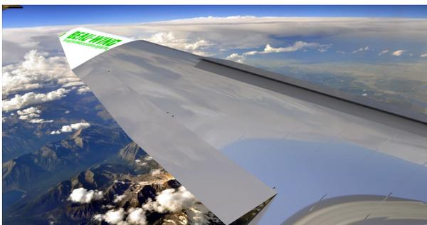
(a) The Airbus A330 wing with a flat extended wingtip.
