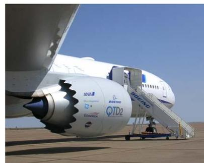
(b) VGC installed on engine.
