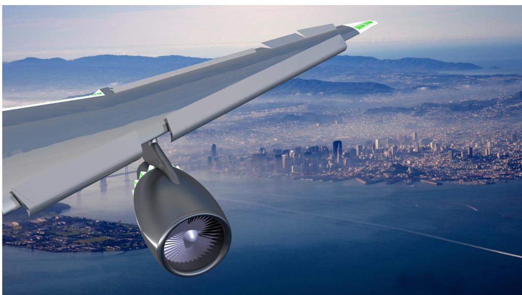
Figure 4.1: The Airbus A330 retrofitted wing with a 90° cant extended wingtip.
