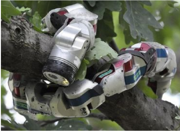
Figure 2.8: Unified Snake: A fixed camera is clearly visible in the head segment. The head provides sensing information [30].
