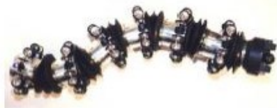
Figure 2.6: GMD-snake2 robot: The second version of the snake-like robots being developed by the GMD group. The robot consists of cylindrical segments with 12 electrical driven wheels around each segment [10].
