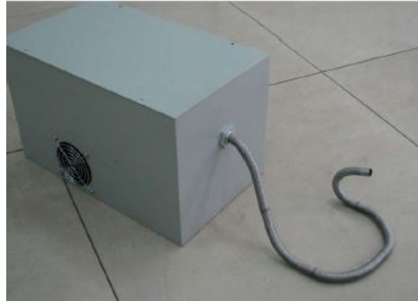
Figure 2.10: Robotic Endoscope: A prototype of a robotic endoscope. As for the HARP, a feeding instrumentation box is visible in which the motors drive the tensioning cables [33].
