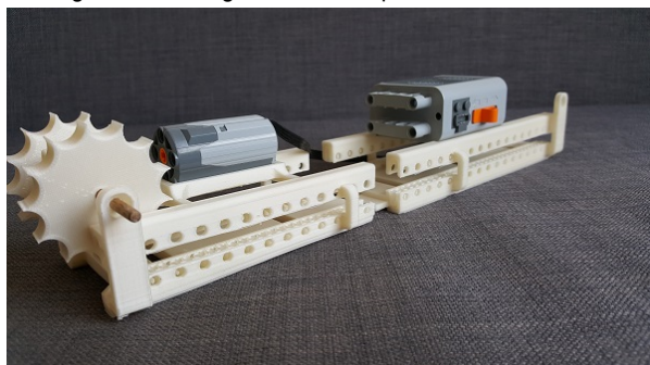
(b) Concept 2: two sprocket wheels as both belt end guidance and belt drive, belt mid guidance by two rows of wheels along the frame.
