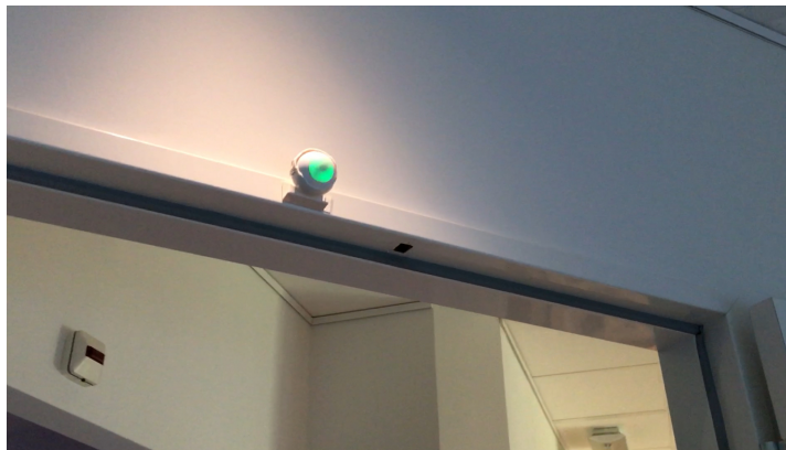
Figure 5.2: A Fibaro motion sensor positioned in the bedroom at the Experience Lab
