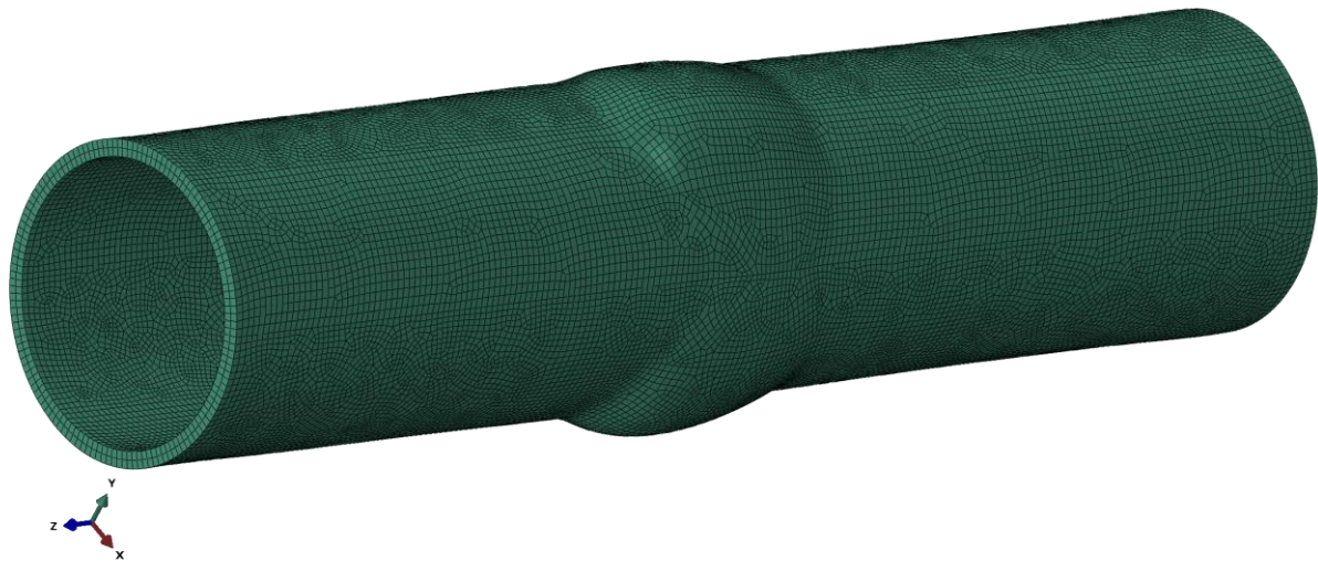
Figure 2-14: Formed Conduit mesh.
