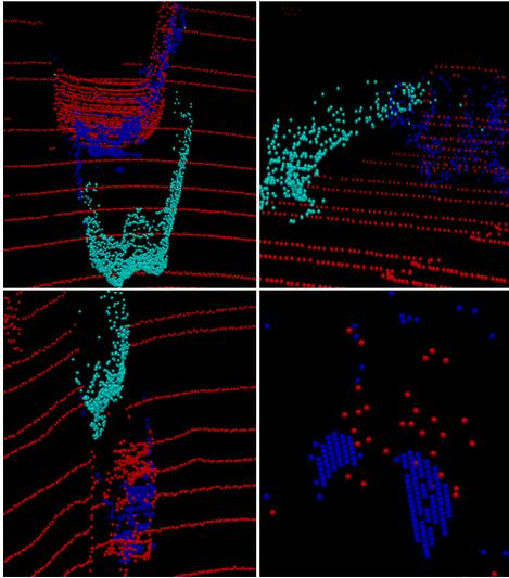
Fig. 10: Localization provided by point cloud from RAID (blue) vs. point cloud generated from monocular depth (cyan) vs. LiDAR point cloud (red) for two cars (top row), a cyclist (bottom left), and two pedestrians (bottom right) visualized in arbitrary view points. RAID matches the ground truth LiDAR point clouds significantly better than the monocular depth based point cloud.
