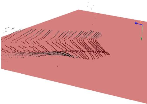
Fig. 11: Ground plane estimation using a LiDAR point cloud and a semantic mask. The orthogonal axes represent the position and orientation of camera fitted on the ego-vehicle. The visualized point cloud is “extracted” by keeping only the LiDAR points that fall on pixels with the semantic class “road” when projected onto image plane. The red plane represents the RANSAC-fitted ground plane using the extracted set of points.
