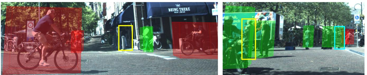
Fig. 4: Detection performance of our proposed method on two busy scenes in the test set. 3D Bounding boxes in red and green show successful detections of cyclists and pedestrians respectively. Yellow boxes indicate where instances are not detected (False Negative), while the cyan box on the right highlights a false detection (False Positive).
