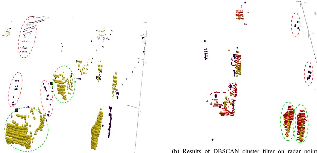
(a) LiDAR points in a scene corresponding to specific instances of interest. Yellow points represent the retained clusters after DBSCAN while those in black are outliers. For two car instances on the left, points highlighted in dotted green ellipses indicate the retained points after filtering while ellipses in red indicate the occluded points in image view that are now filtered out.
