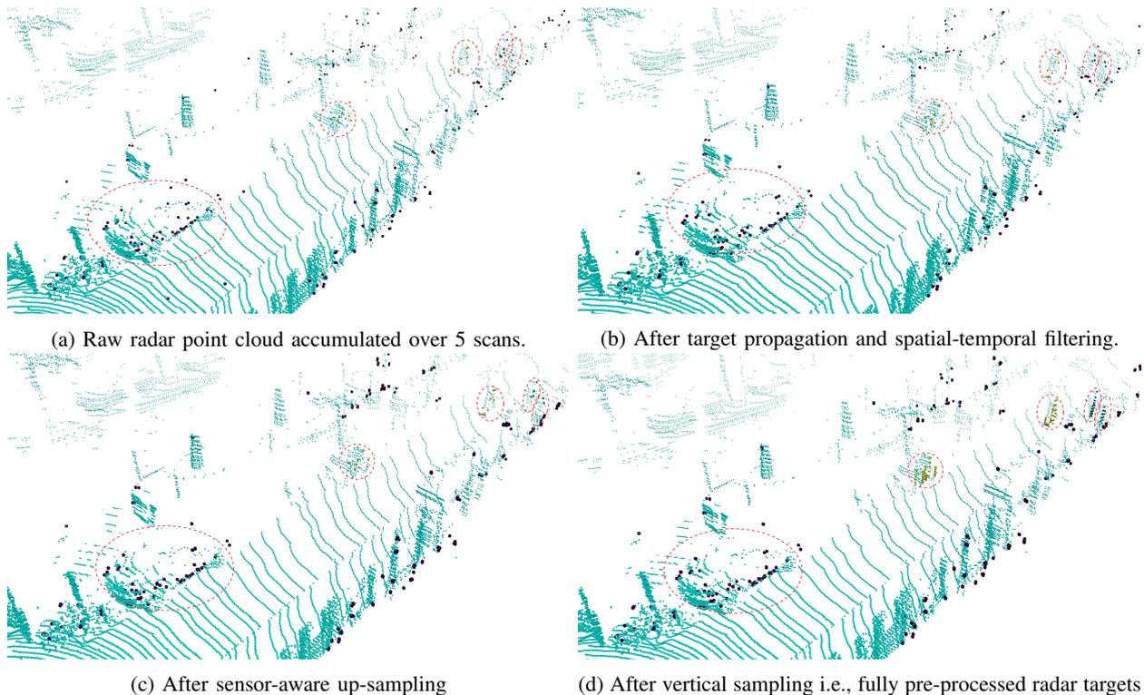
Fig. 7: Radar point cloud visualization at various stages of pre-processing. Points in cyan represent LiDAR points to comprehend the scene context. Radar targets are colored based on the compensated Doppler value. Note that the cyclists and pedestrians are moving while the car is parked (all the instances are highlighted in dotted ellipses).
