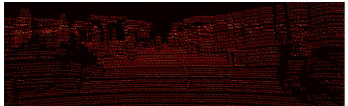
(a) Raw LiDAR point cloud projected onto the image plane
