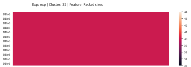
Figure 16: Heatmap showing the fixed packet size in a different DDoS cluster
