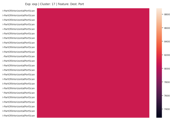
Figure 14: Heatmap showing the continual use of the same destination port in a horizontal port scan cluster
