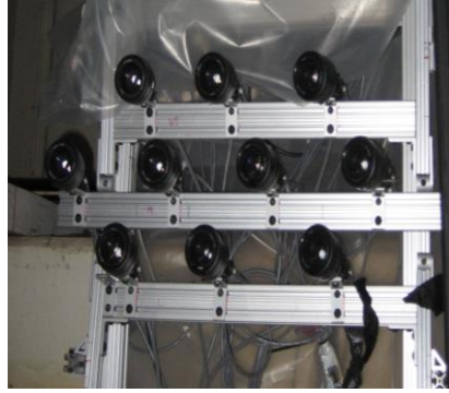
Figure 1 Ten-camera array of Flea 2 model FL2-08S2M/C from Point Grey Research, Inc. CCD cameras, with 50mm Nikkor lenses, typical of those used for the experiments presented herein.
