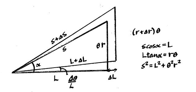
Fig 2 hinearization of the strains Part of helix layed flat
