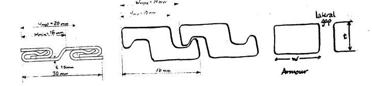
Fig 1 Components of a nonbonded flexible pipe
