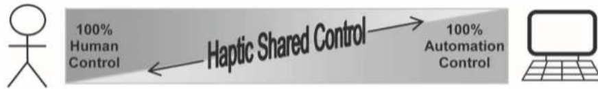
Figure 2.3: Haptic shared control facilitates the communication of authority between human and automation from fully automated to full manual control [6] [7].
