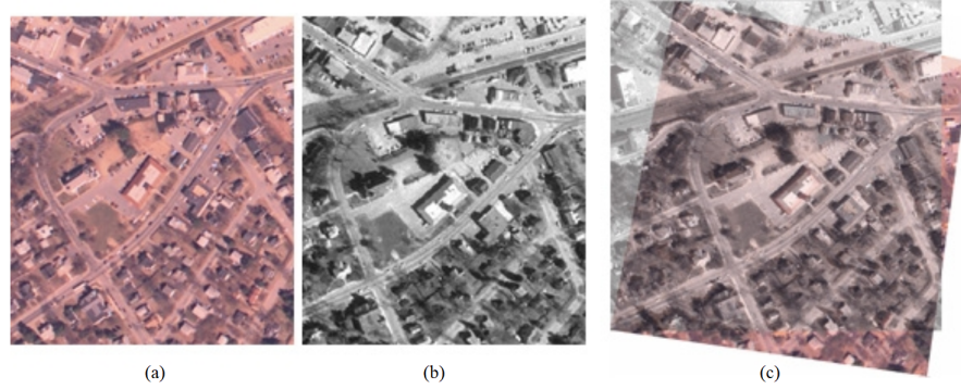
Figure 2.11: (a) and (b) Images containing common visual information, but retrieved from different viewpoints. (c) The registration result of (a) and (b). (Figures: MATLAB Tutorials).
