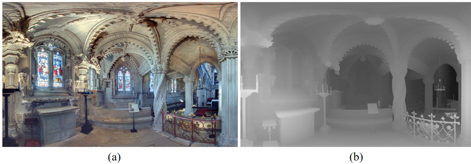
Figure 3.6: a) An image with intensity values in RGB colours. b) The depth image of Figure (a) in grayscale. (Figures from NCTech [2018].)
