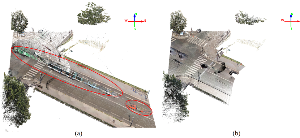
Figure 2.4: a) Point cloud square tile of 250m^2 in which moving objects (cars) have been scanned. These are circled in red. b) Point cloud square tile of 250m^2 representing the same area as (a) in which moving objects have not been scanned.
