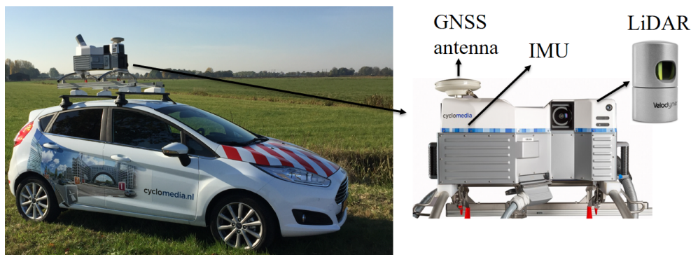
Figure 1.1: A Light Detection And Ranging (LiDAR) sensor, a Global Navigation Satellite System (GNSS) receiver and an Inertial Measurement Unit (IMU) deployed on a mobile platform for the purpose of street view geo-referenced laser scanning. The Figure depicts a MLS system as configured and mounted to a vehicle of the company CycloMedia Technology B.V.
