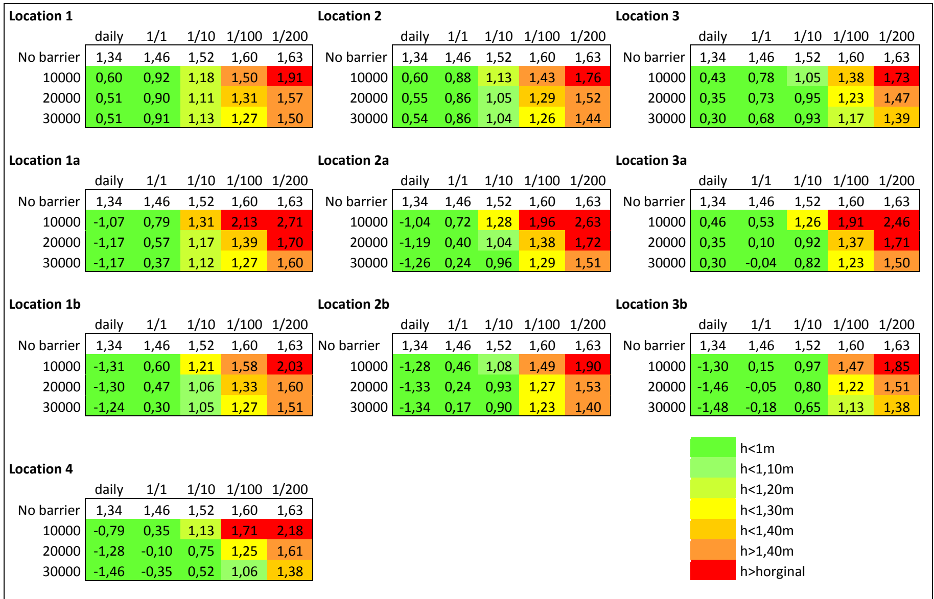
Figure M-3: results for a discharge sluices at 10 locations for 3 opening sizes and 5 design river discharges, 2010
