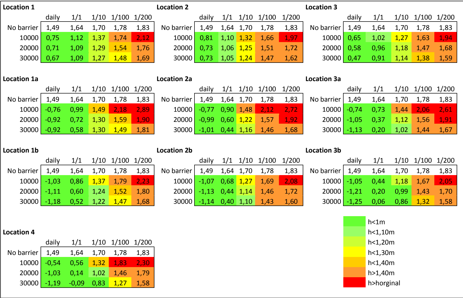
Figure M-4: results for a discharge sluice at 10 locations for 3 opening sizes and 4 design flood waves, 2050
