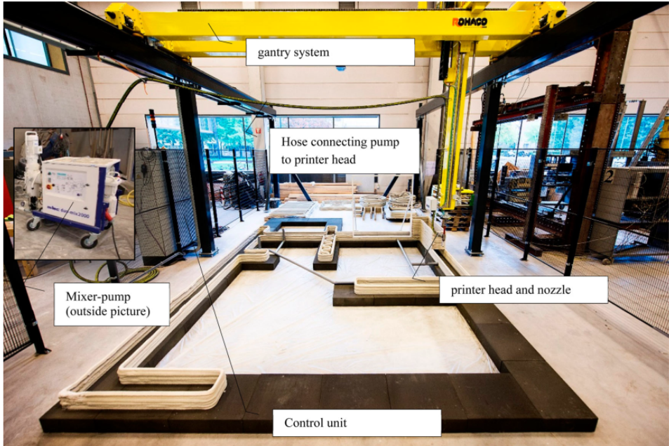
Figure 2.7: 4 DOF gantry-based system, adapted from [35]
