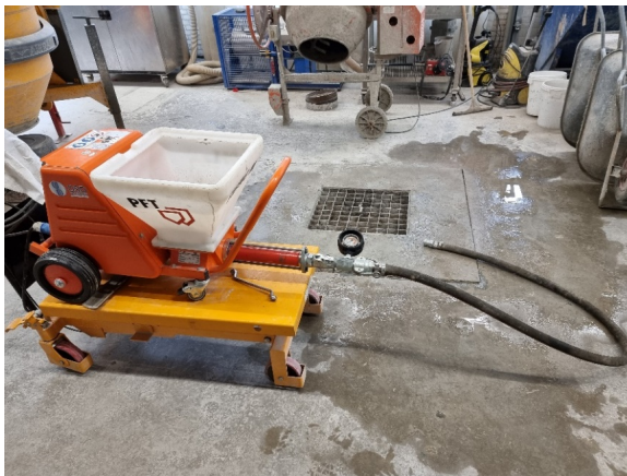
Figure 3.5: A PFT SWING-M conveying pump and the hose
