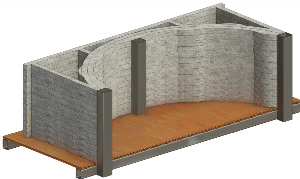
Figure 6.17: A 3D view of three locations where the steel frame connects to the 3D printed bridge
