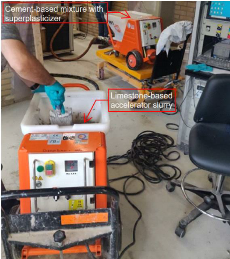
Figure 4.3: Two PFT Swing-M conveying pumps with separate mixtures and hoses [40]
