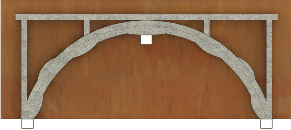
Figure 6.15: Top view of the 3D printed bridge on the steel frame structure
