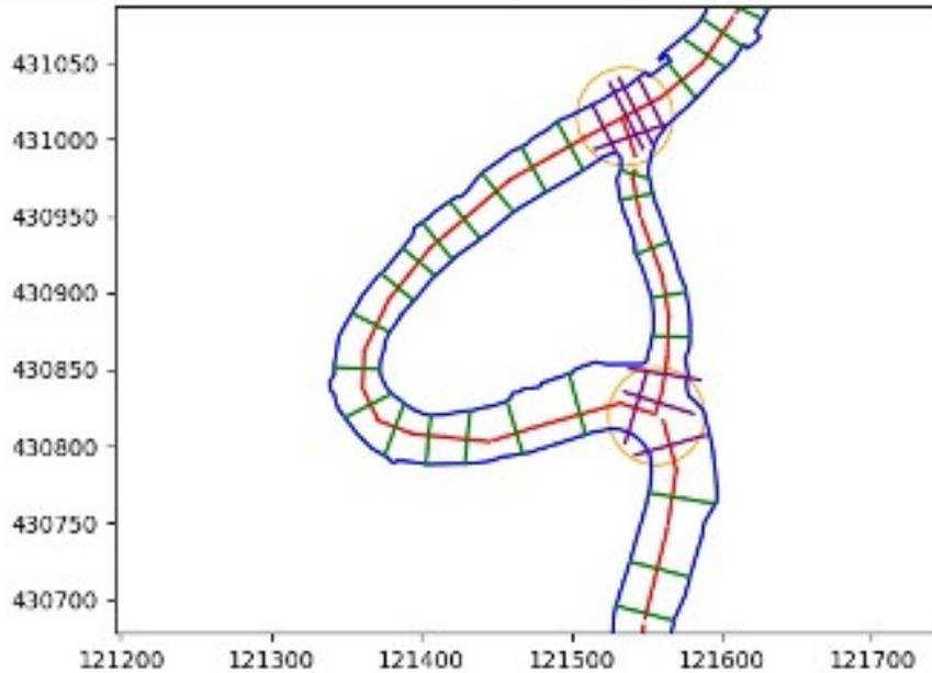
(b) The approximation of the channel width near junctions of channels
