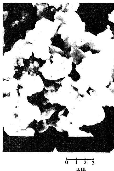
Fig. 6. SEM micrograph of a completely converted Ti particle. Swelling during nitridation is observed.
