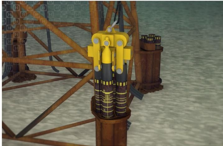
Figure 2.5: Push-in pile foundation including hydraulic installation tool
