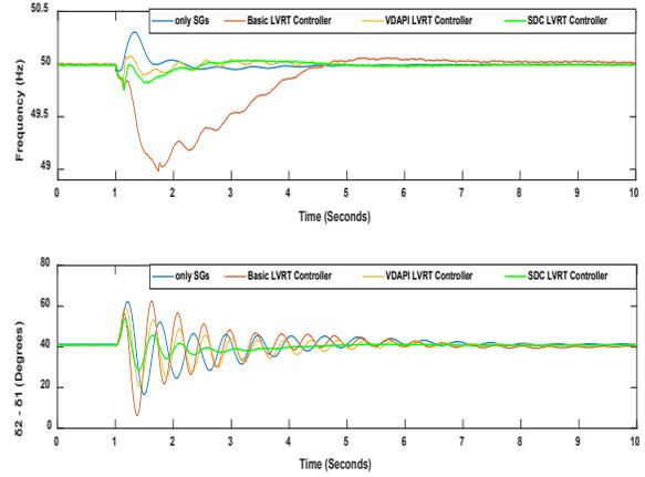
Figure 8. 52% WG share Frequency & Rotor angle responses
