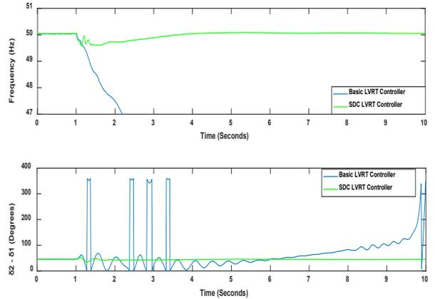
Figure 9. Frequency & Rotor angle responses with 75% WG share
