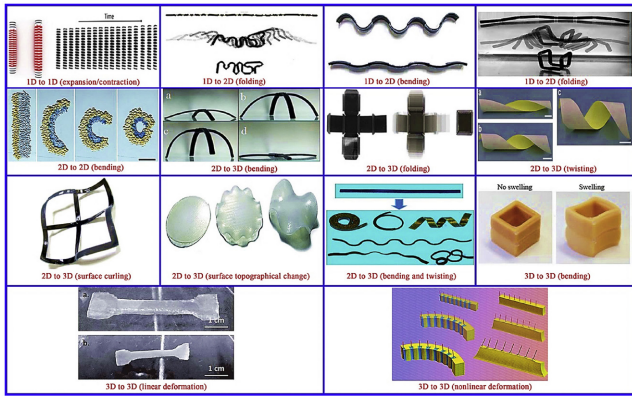
Figure 17. Different ways of shape change for 4D printing (Mallakpour et al., 2021).
