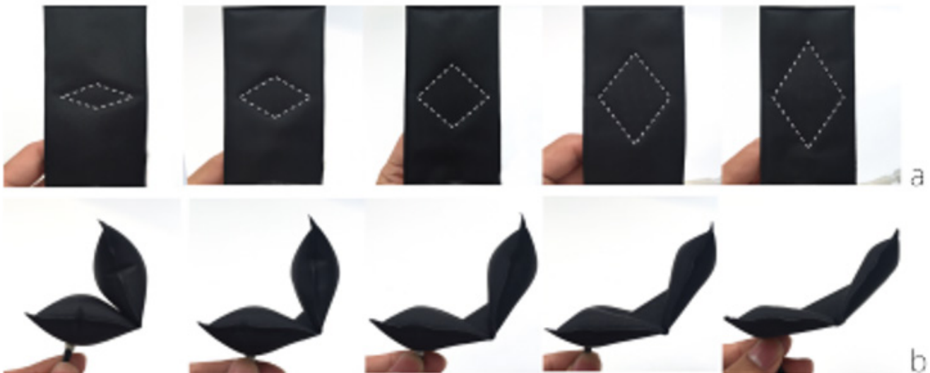
Figure 68. The width/height aspect ratio of the diamond hinge (a) determines the bending angle at full inflation (b) (Out et al. 2016).
