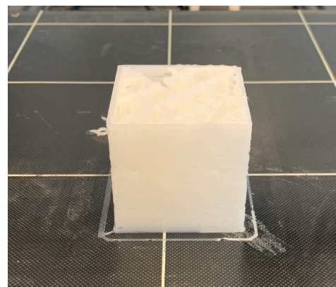
Figure 37. Result after buying new TPU (BASF Ultrafuse TPU 85A). The print remained attached to the bed throughout the entire process.
