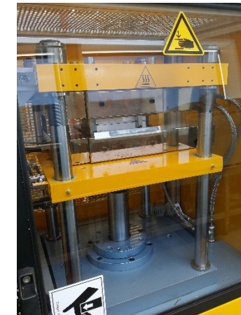
Compression moulding process
