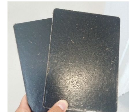
EPS coated flax fibre ( 30 wt.% ) based composite panels
