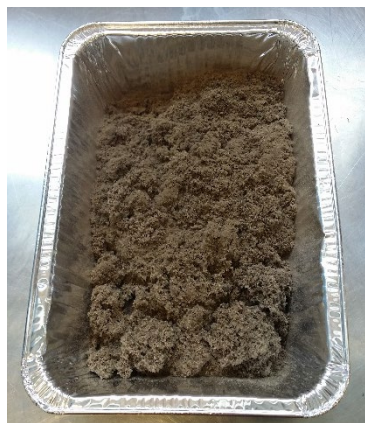
Short fibres after grinding
