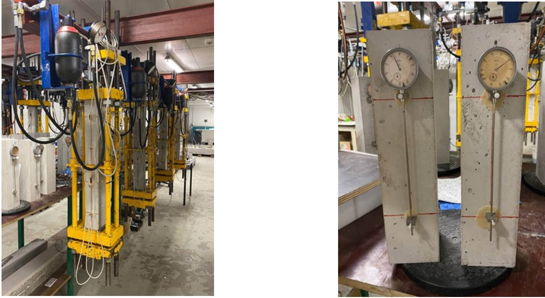
Figure 4.2 Photos of the ongoing creep test (left) and shrinkage test (right).
