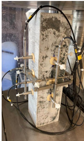
Figure 3.4 Elastic modulus test. The changes of the specimen dimensions during the loading process were measured precisely. For this purpose the linear variable differential transducers (LVDTs) were aligned vertically on the four sides of the concrete prism.
