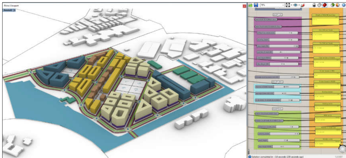
Figure 21. Example of the Graphical User Interface of the parametric modelling tool in Rhinoceros/Grasshopper. On the left, 3D visualization in the Rhinoceros viewport. On the right, the Grasshopper window with information panels and data nodes.
