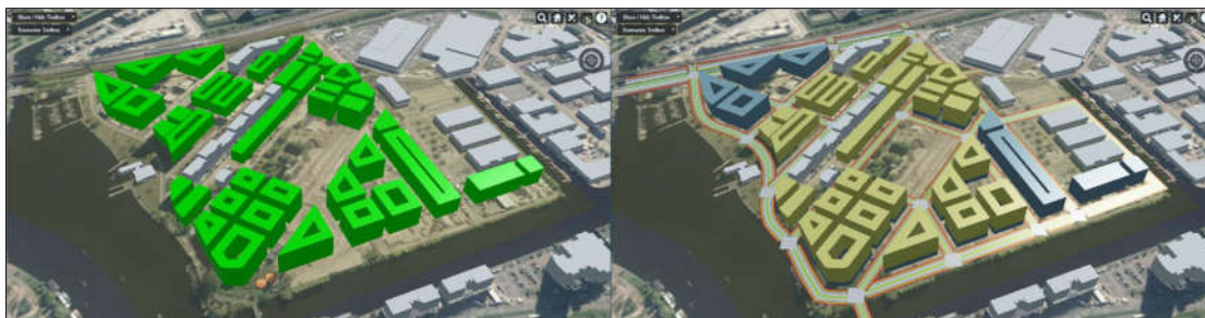
Figure 8. Example of the online scenario visualization interface: Scenario B of Figure 7 is presented here visualizing either the new buildings (in green) (left) or the new usage zones (right). Existing buildings are visualized in white.
