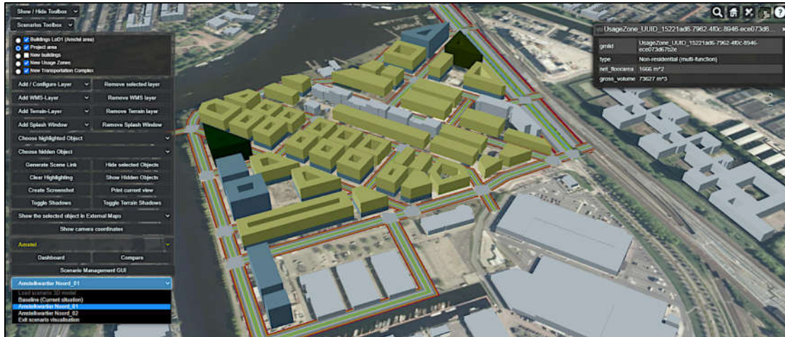
Figure 24. Visualization in CesiumJS of a scenario via the extended graphical user interface of the 3DCityDB web-map client.
