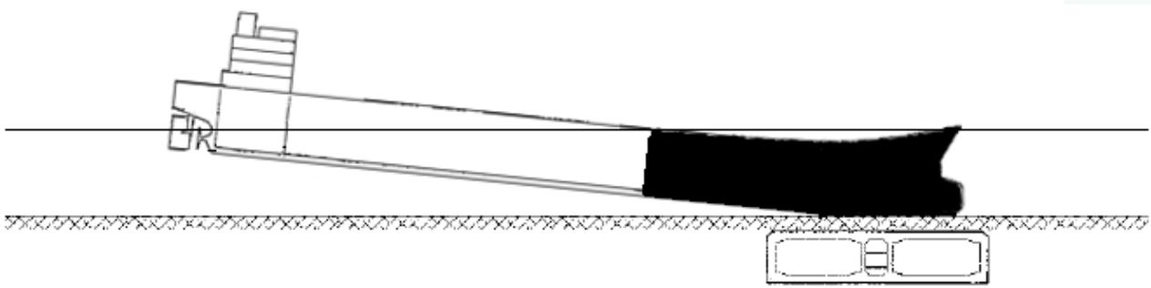
Figure 37 – Option 2: prow deforming plastically
