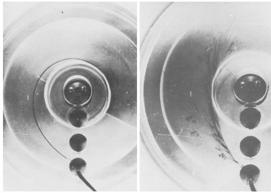
(a) Laminar flow (b) Turbulent flow Figure 2.3: Secondary flow in a cone plate rheometer,[19]
