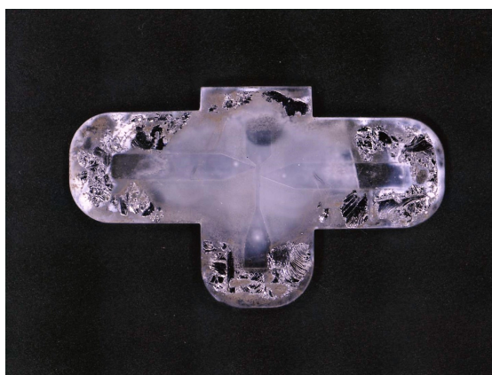
Figure E.12: Picture of PMMA being released with Isopropanol.
