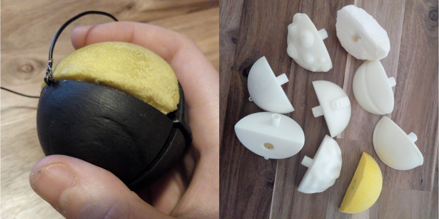
Figure 6.5b: The printed prototype, on the left the one painted in conductive paint and connected to the arduino, on the right the different talent quarters unpainted.
