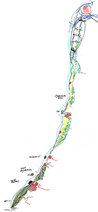
4.20 Sketch of the Dutch coastline sometimes maintained, sometimes reinforced, sometimes extended seawards and sometimes further reinforced on the landward side.
