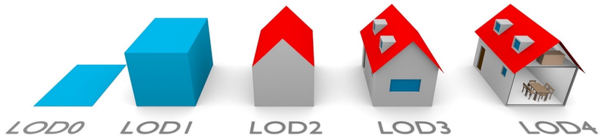
Figure 1.2: A visual example of the refined LODs for a residential building [Biljecki et al., 2016].
