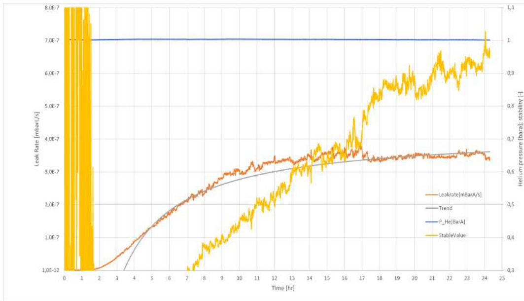
Figure 5.13: Measured leak rate [mbarL/s] and helium pressure [bara] of specimen 10793-6
