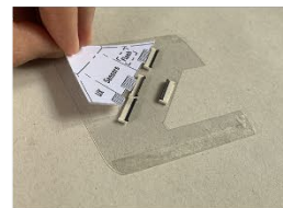
Slide contact pads of transferred Modules in FPC connectors of new 5G Advanced NETWORK Module upgrade
