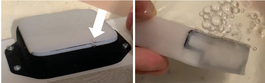
Figure J4: (a) bubble appearing from exterior mounting variant (b) continuous stream of bubbles in interior mounting variant
