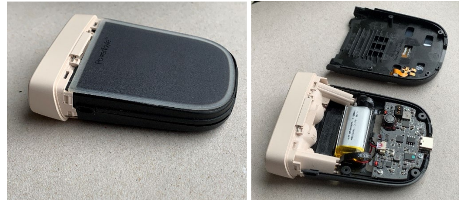
Figure I3: (a) No ‘direct access’ design due to inner enclosure sandwich design; inner structural part necessary for provide support to the flexible PV panel on one side and button and LEDs on the other. (b) unscrewing the enclosure parts unlocks the earphone charging cradle part. LiPo battery is fixated using double sided adhesive tape.
