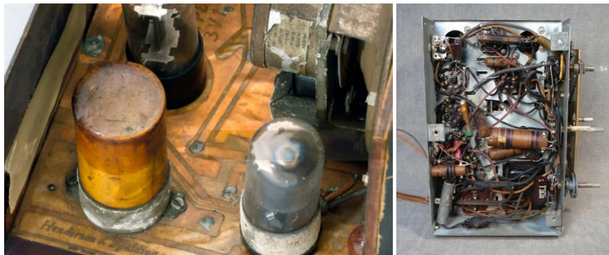
Figure F2: (a) Paul Eisler 1942 radio with PCB, (b) GE radio from 1937 with point-to-point wiring
