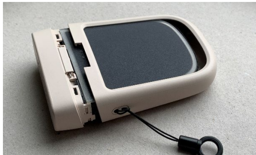
Figure I2: Notably hard to open without damage due to snap fits on four sides; no flexible sealing of PV panel, but pressed to the outer enclosure through the wedge design
