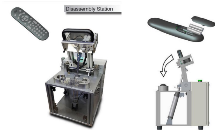
Figure 17: Disassembly station for a TV remote (D'Andrea & Evers Design)
