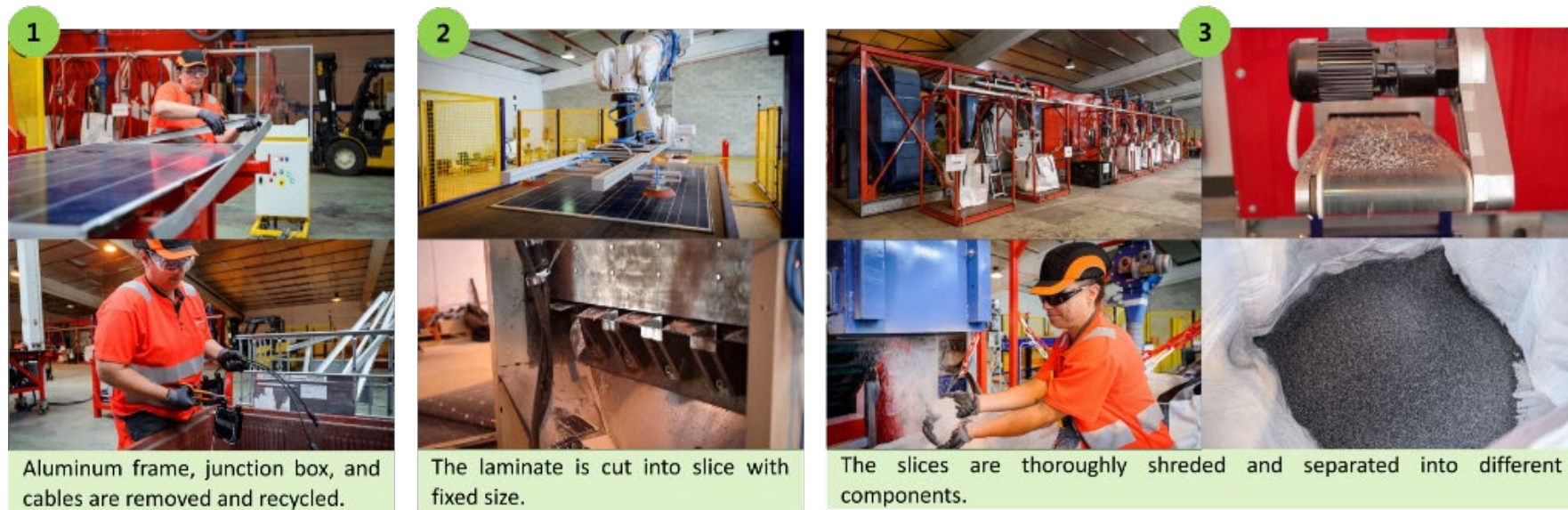
Figure C11: PV recycling process by Veolia
