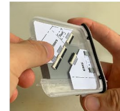
Assembly of upgraded PCBA in drawer for testing
