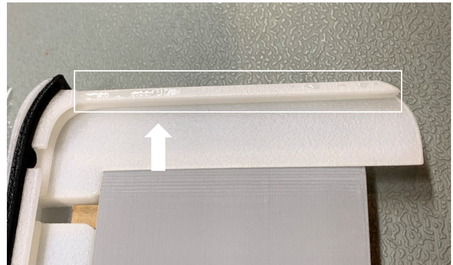
Figure 79: Droplets remain on the rail after removal of the drawer after the mounting variant underwent a IPX7 test
