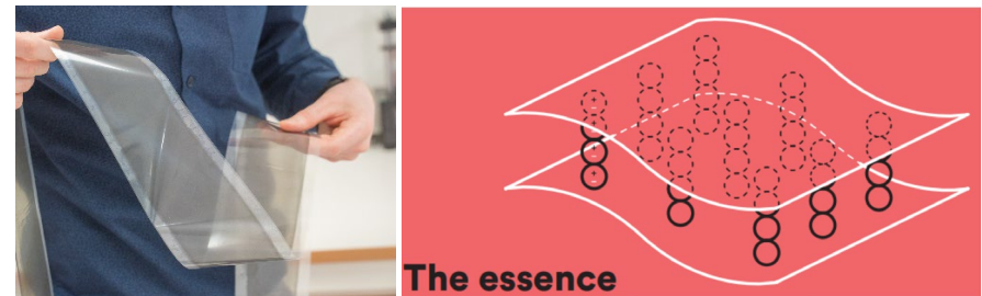
Figure 23: (a) Anisotropic conductive adhesive film with (b) traces formed in z-direction through a magnetic field
