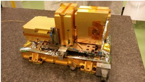
**Figure 4.19:** The ISA, three instruments aligned along different axes, mounted onto a baseplate.
