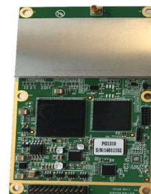
**Figure 4.17:** GSD800 GNSS Receiver [30]
