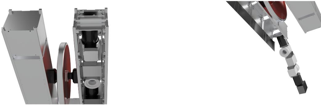
**Figure 6.6:** Boom deployment mechanism, stowed and deployed
