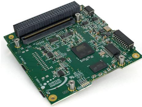
**Figure 6.26:** The On-board computer from ISISPACE, which will be used in the spacecraft [94]
