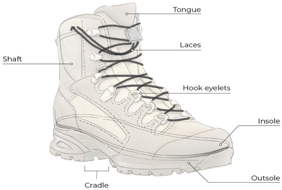
Figure A3.2 - Army boot parts
