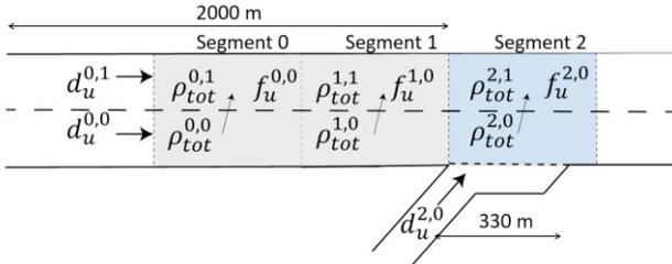
Fig. 2. 2-lane mainline carriageway with an on-ramp
