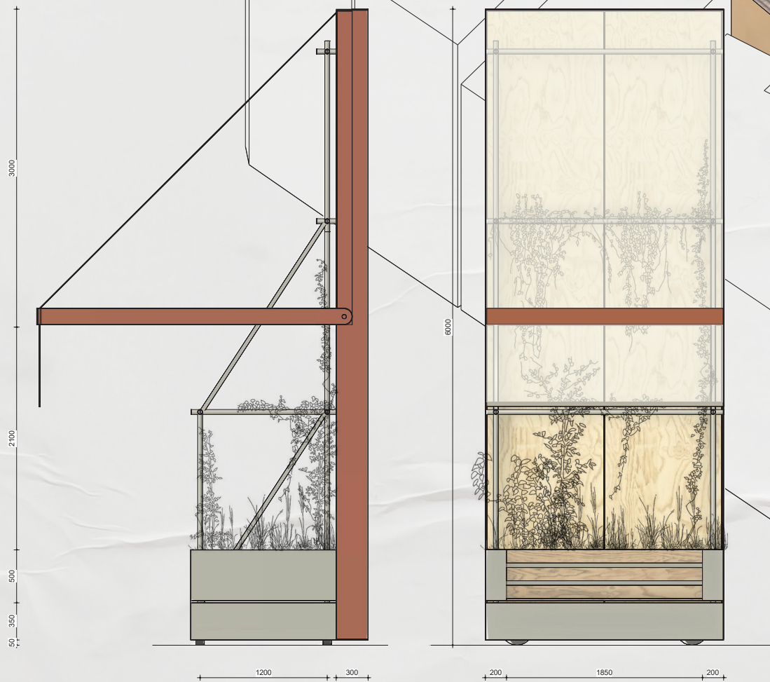
1:20 elevations (scaled to 1:50) showing the retractable canopy
