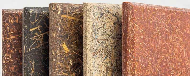
Bio-composite panels, made out of 33% reed, 33% chalk, and 33% bio-based resin
