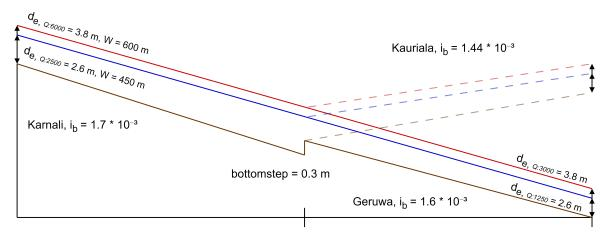
Figure 6.2: Initial longitudinal profile of the system. Section slope, width and corresponding equilibrium depth are added.
