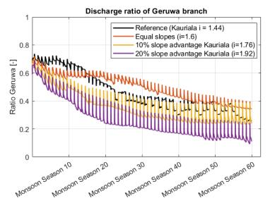
Figure 7.15: Discharge distribution with different slope of Kauriala branch.
