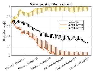
Figure 7.5: Discharge distribution with varying spiral flow intensities.
