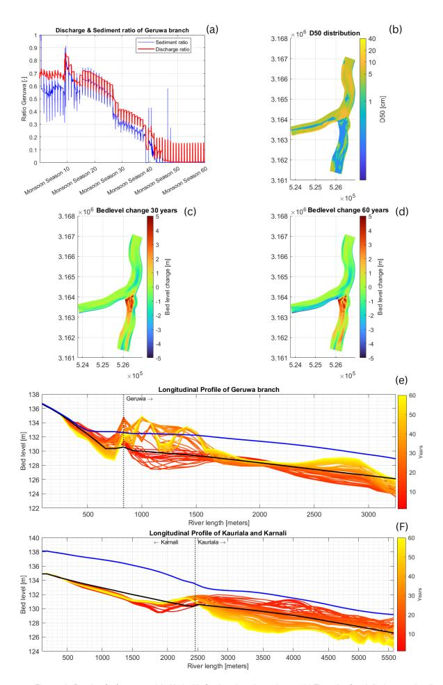
Figure 7.3: Results of reference model with double flood peak on the tenth year. (a) The ratio of total discharge and sediment flux entering the Geruwa branch. (b) Sediment grain size distribution of the bed surface after the simulation period. (c) and (d) Cumulative erosion and deposition after 30 and 60 years. (e) and (f) the longitudinal profiles of all three branches and their development during the simulation period.
