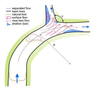
Figure 3.4: Schematic of processes at a bifurcation located near a river bend. Note the Bulle effect near the entrance of the offtaking channel. Arrows indicate the flow patterns influenced by the secondary flow. Figure adopted from (Kleinhans et al., 2013; van Denderen et al., 2018)
