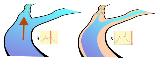
Figure 5.3: Conceptualised sediment flux and deposition during peak flood event (left) and during low flow conditions (right).
