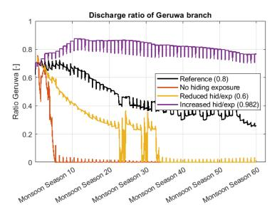
Figure 7.12: Discharge distribution with different Hiding/Exposure coefficient, see Eq. (A.14).
