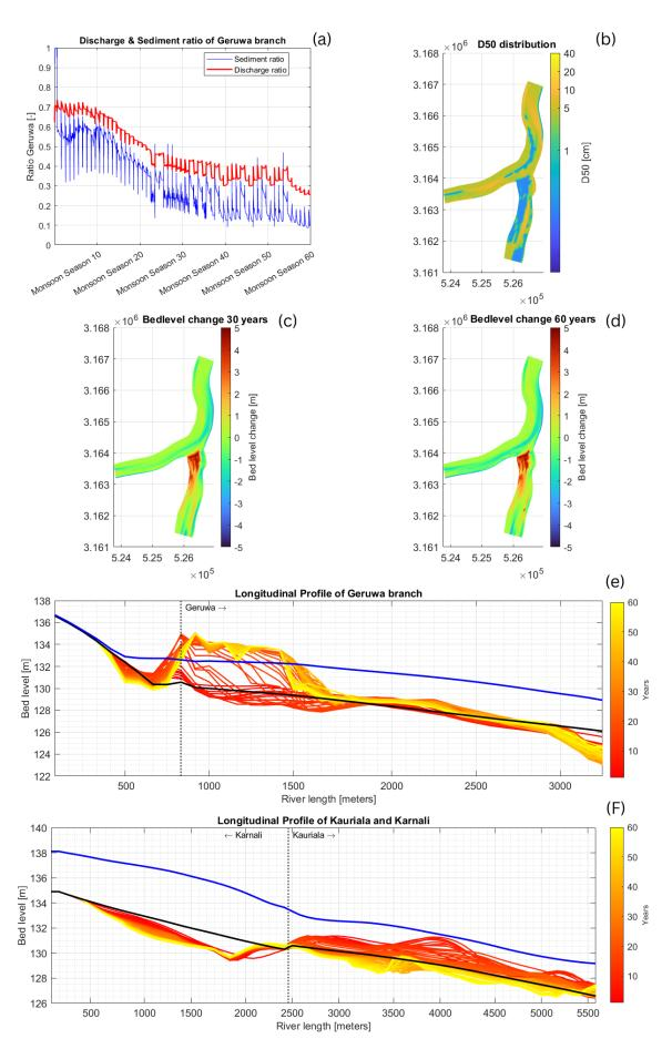
Figure 7.1: Results of the reference model. (a) The ratio of total discharge and sediment flux entering the Geruwa branch. (b) Sediment grain size distribution of the bed surface after the simulation period. (c) and (d) Cumulative erosion and deposition after 30 and 60 years. (e) and (f) the longitudinal profiles of all three branches and their development during the simulation period.
