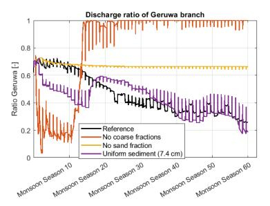
Figure 7.14: Discharge distribution with different sediment compositions.
