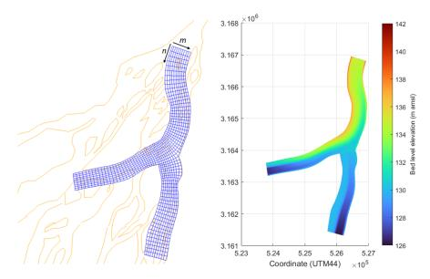
Figure 6.1: Left image shows the computational grid overlayed on the Karnali land boundaries (October 2023), m and n directions are shown. On the right, the initial bathymetry of the reference model is shown.
