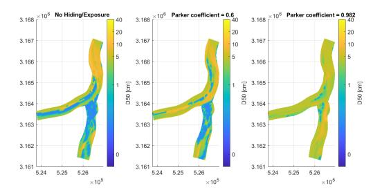
Figure 7.13: D50 distribution of the model runs with hiding/exposure coefficients.
