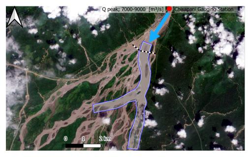
Figure 6.4: Model Domain on top of Sentinel image from 11-09-2019 when 2790  $m^3/s$  was measured at the Chisapani gauging station.
