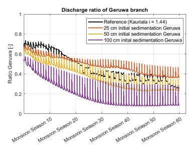
Figure 7.16: Discharge distribution with different amounts of bed level increase of the Geruwa branch.
