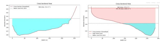
Figure 4.6: Cross sections; (left) KAR1, three kilometres upstream of the bifurcation. (right) Location BIF3, right before the bifurcation, located in the bend, see the white dotted line in Fig. 4.3.
