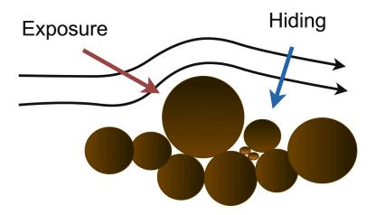
Figure 3.1: Hiding/Exposure effect, redrawn from Scheer et al. (2002).
