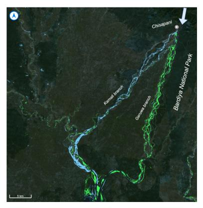
Figure 1.4: Map of the Karnali river changes downstream of Chisapani between 2000 and 2023. Green pixels show where surface water has been turned into land (accretion, land reclamation, droughts). Blue pixels show where land has been changed into surface water (erosion, reservoir construction). Picture created with the Aquamonitor tool (Donchyts et al., 2016).
