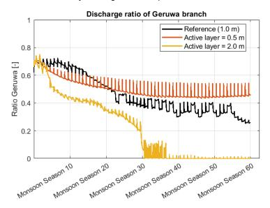
Figure 7.10: Discharge distribution with different active layer thickness.
