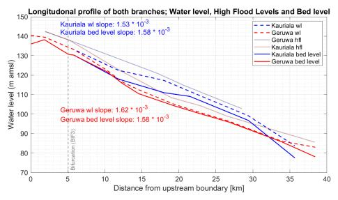
Figure 4.7: Measured water level and slope extraction in both bifurcates of the Karnali. The semitransparent lines indicate the high flood level in the locations where it could be identified by either markings from the waterboard or asking the local inhabitants. Bedlevel points were retrieved from the deepest point of the measured cross-sections.
