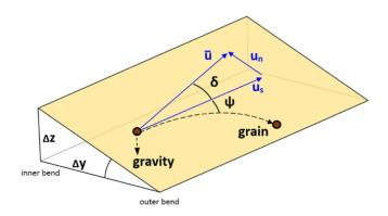
Figure 3.3: Drawing showing particle deflection due to transverse bed slope gravity pull and secondary flow. The trajectory of sediment particles travelling in the direction  $\vec{u}$ , are deflected downslope ( $\psi$ ) due to gravity pull and upslope due to secondary flow ( $\delta$ ). Figure adopted from (Baar et al., 2018).
