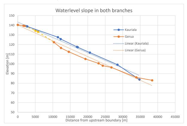
Figure 8: The slope of the measured water levels along the Kauriala and Geruwa branches. The upstream boundary is the most upstream data point. Note the yellow, dashed line represents the measured point at location BIF3, the only location where the RTK GPS did not have a fixed signal and where we had to rely on a DGPS signal with poor accuracy of a couple of meters
