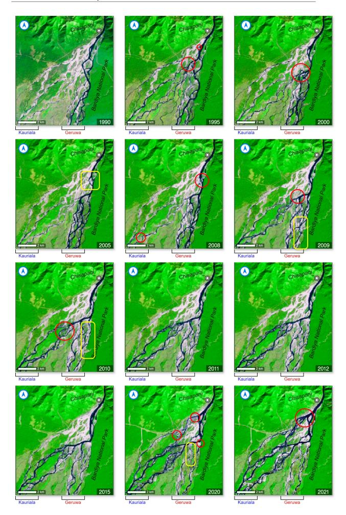
Figure 4.1: Recent history of the Karnali bifurcation (1990-2021) Landsat 7 SWIR composites after monsoon period (Oct-Dec), Notable erosion events or channel activations are highlighted with red circles and sedimentation with the yellow rectangle.
