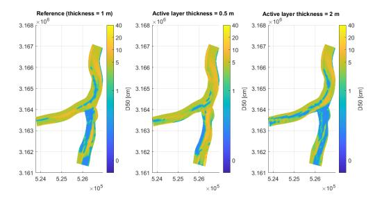
Figure 7.11: D50 distribution of the model runs with various active layer thicknesses.
