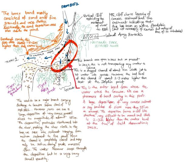
The third major bifurcation point and most crucial for the supply of the Geruwa branch. Entry to the Geruwa branch is completely blocked by a deposition of large boulders. Efforts by the national park authorities to dredge a channel through the blocked entrance seem insufficient to reestablish the at around 1-1.5 meters deep, far less than the depth of the main channel at 4 m. Sediment size on the inner bend is significantly smaller than in the outer bend.
