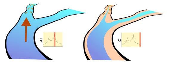
Figure 4.4: Conceptualized sediment flux and deposition during peak flood event (left) and during low flow conditions (right).
