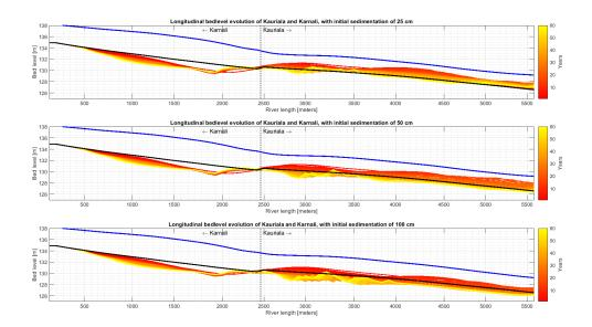
Figure 7.17: Bed level evolution of the Kauriala branch at different initial sedimentation of the Geruwa branch.
