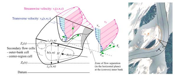
Figure 3.2: Drawing of the flow profiles that occur in a river bend. The flow directed to the inner bend near the river bed and the flow directed to the outer bend near the water surface cause the secondary flow, combined with the streamwise flow the river experiences a helical flow. Figure adopted from (Blanckaert, 2011). (right) Drawn streamwise velocity profile in the Karnali bifurcation (BIF3). The zone of flow separation at the inner bend is indicated with the orange line.
