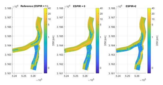
Figure 7.6: D50 distribution of the model runs with different spiral flow (ESPIR) magnitudes.
