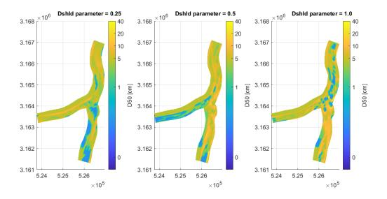
Figure 7.9: D50 distribution of the model runs with Dshld coefficient values
