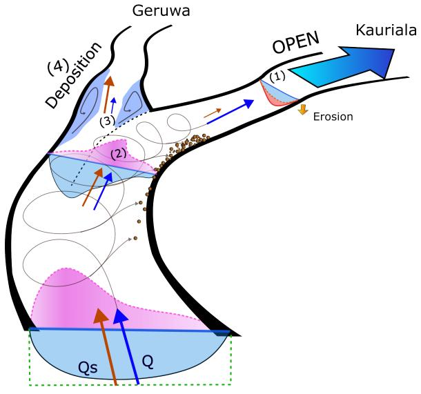
Figure 5.4: Processes involved in hypothesis two. The streamwise velocity profile is shown in pink, and the areas of flow separation are shown in dark blue. Spiral flow is shown and the size of the arrows represents the magnitude of the discharge and sediment flux.
