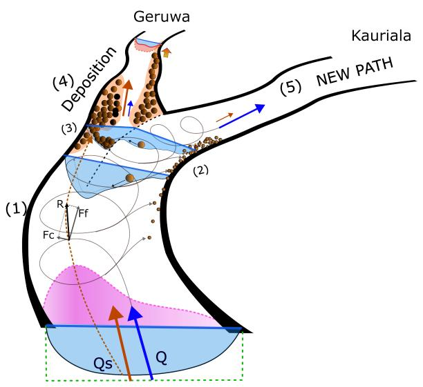
Figure 5.2: Processes involved in hypotheses two. The brown patches with sediment particles show deposition. Spiral flow is shown and the size of the arrows represents the magnitude of the discharge and sediment flux.
