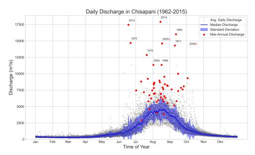
Figure 2.1: Hydrograph from the Chisapani gauging station
