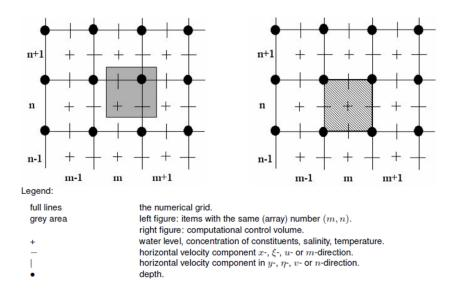
Figure A.2: Computational grid and components. Image retrieved from Deltares (2018)
