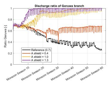
Figure 7.7: Discharge distribution with Ashld parameter values.
