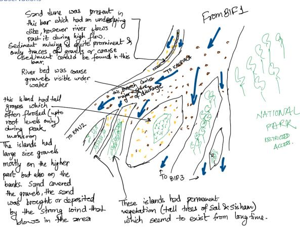
First bifurcation point of the river. The western bank consist mainly of sand due to intake structure of the irrigation channel just upstream of the point. Some gravel and boulders are present on top of the sand. The first large bar (0.260 km²) that starts to split the Karnali channel consists of coarse gravel and boulders and has little grasses in the middle. The other large, more stretched out bar to the west is covered in multi year vegetation.
