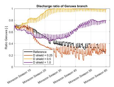
Figure 7.8: Discharge distribution with various Dshld parameter values
