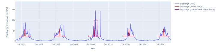
Figure 6.3: Discharge, Chisapani gauging station data and model input simplification, from 2009 and surrounding years. Note the two distinct peaks of high intensity.
