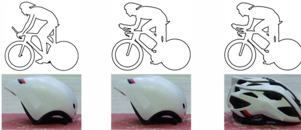
Figure 3. Riding configurations and helmets used. Upright position with aerodynamic helmet (left). Time trial position with aerodynamic helmet (middle). Time trial position with conventional road helmet (right).
