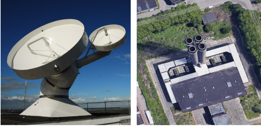
Figure 7.11: PARSAX (left) and measured industrial chimney at approximately 1185 meters from the radar sensor (right).
