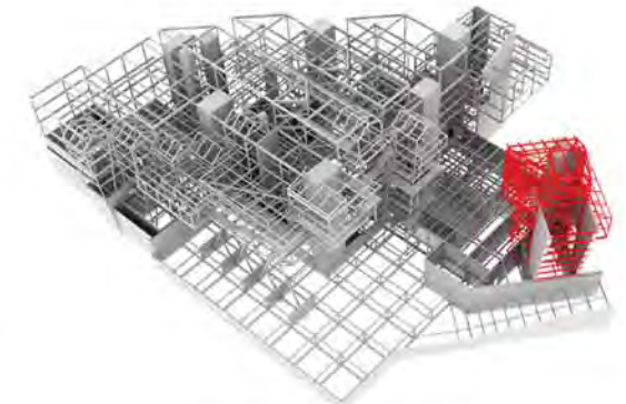
10. Self-Standing Structure with Concrete Structural Base.
