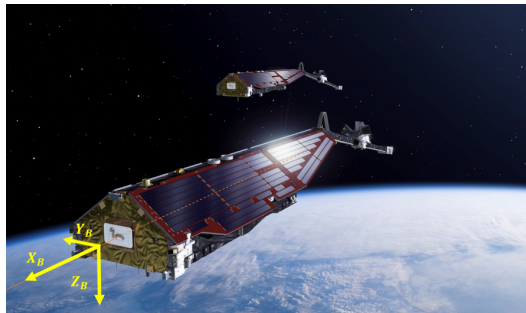
Figure 5.4: Swarm (courtesy: ESA). The satellite body-fixed coordinate system is shown in yellow.
