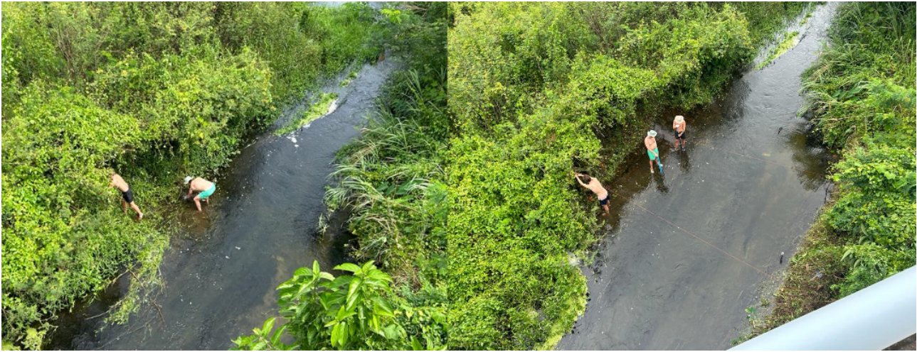
Figure 2.7: River B.11: the plants were cleared and the cross-sections were measured
