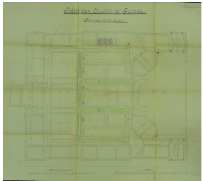
9. Plan of the basement with steam heating, Rud Otto Meyer - DPW
