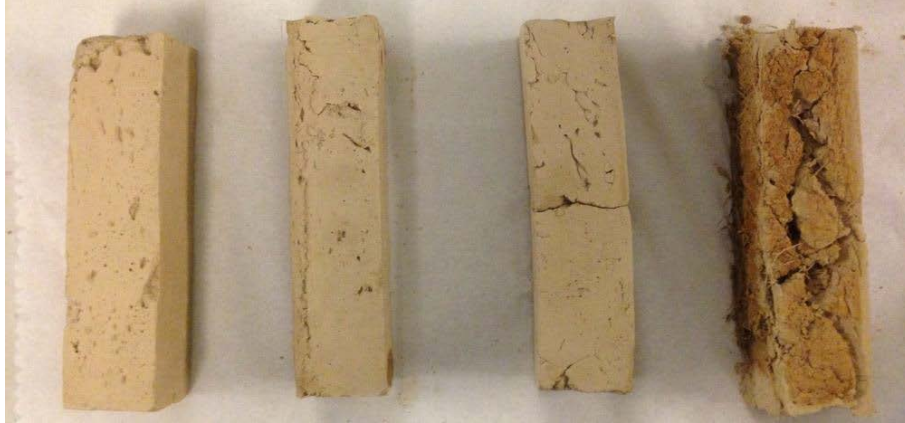
Image 12: Loam brick samples removed from mould. From left to right: loam; ALE, Abaca fibre; loam, ALE; loam, commercial alginate, Abaca fibre (Zlopasa, 2015).
