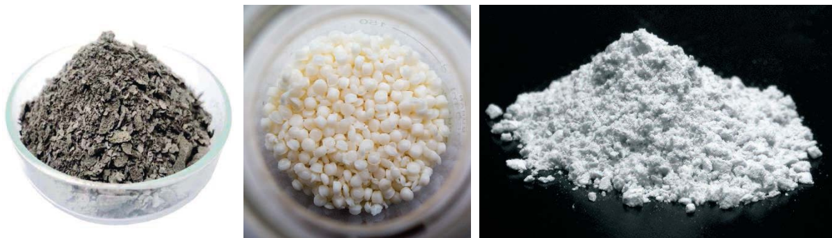
Image 3 to 5: Examples of recycled materials produced by wastewater treatment. From left to right: alginate biopolymers, polyhydroxyalkanonate bioplastic and struvite (van Loosdrecht and Brdjanovic, 2014, p. 1453).
