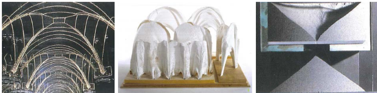
Image: 32-33: Model-making methods devised by Frei Otto. From left to right: Chain net; Plaster bandages; Sand piles (Otto, 1996, p 63-64).
