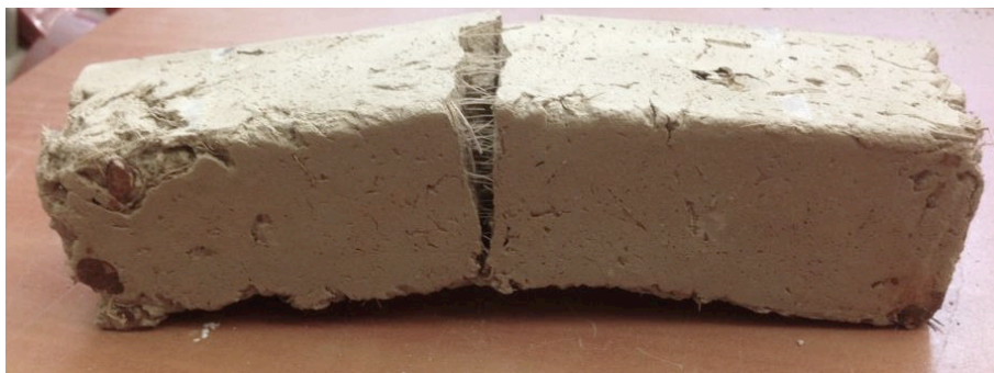
Image 13: Loam brick sample with ALE and Abaca fibres after three point bending test (Zlopasa, 2015).
