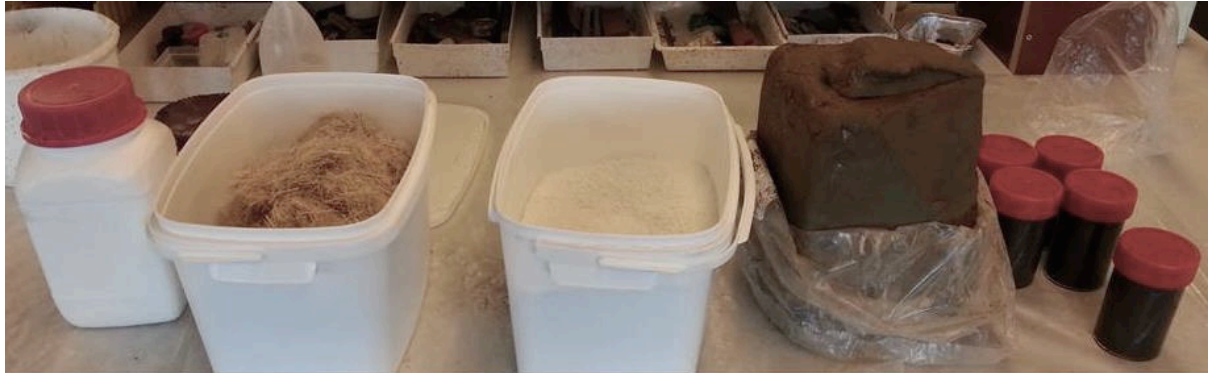
Image 8: Components for brick samples, from left to right: commercial alginate, Abaca fibres, silt, modelling clay, ALE (Zlopasa, 2015).
