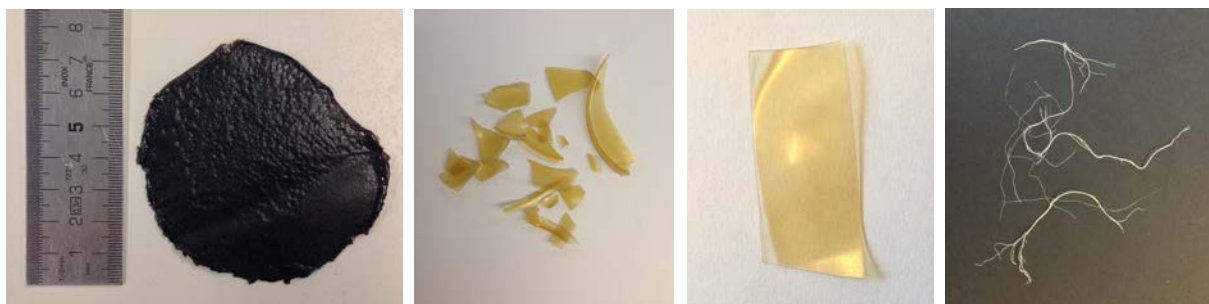
Left, image 18: Pure ALE looks and acts like a black, leather-like, elastic plastic (Own picture).
