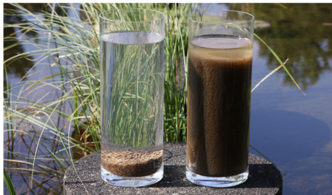
Image 6: Nereda Aerobic Granules (left) next to Conventional Activated Sludge (CAS) (Royal HaskoningDHV b, 2014).
