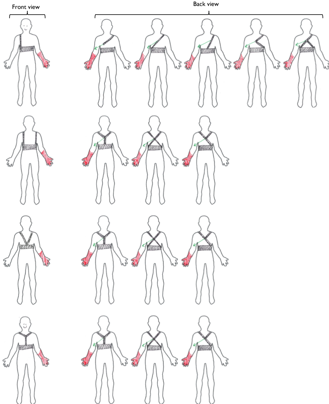
Figure 28. Schematic figures of all the remaining options for the elastic chest strap. The first column shows the various configurations on the front of the body and the rest of the column show remaining configurations on the back of the body for the corresponding row. The amputated arm is shown in red, the straps are shown in black and green the Bowden cable and the arrow pointing in an approximate direction of the activation force.
