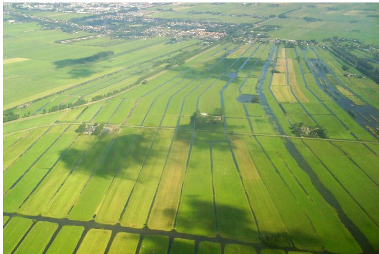
**Figure 1.1:** An aerial photograph of a Dutch polder near the town of Wilnis showing a drainage system with many small ditches.
