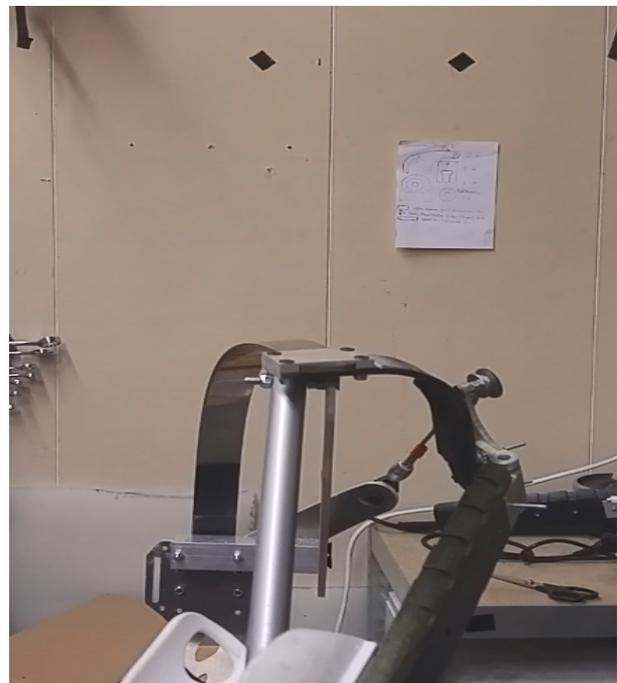
(b) Problem of the first total setup: collision with input arm
