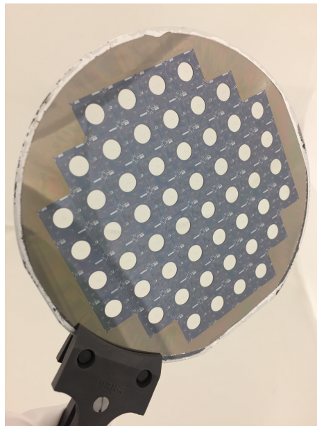
Figure 4.10: Frontside of the wafer after PDMS membrane release.
