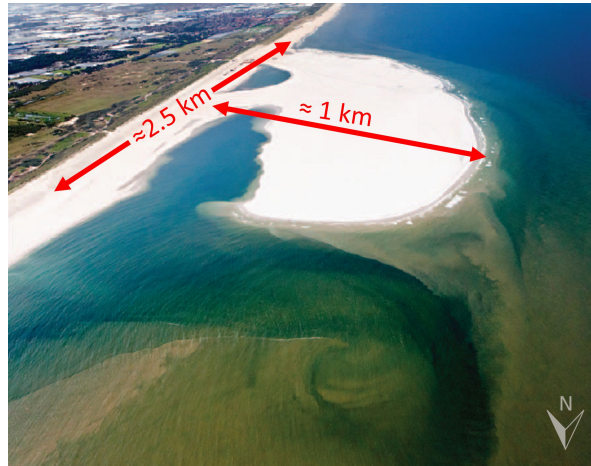
Figure 1: Aerial photograph of the Sand Motor after completion (September 2011). Note the clouds of fine-grained material moving to the North. Picture courtesy of Rijkswaterstaat / Joop van Houdt
