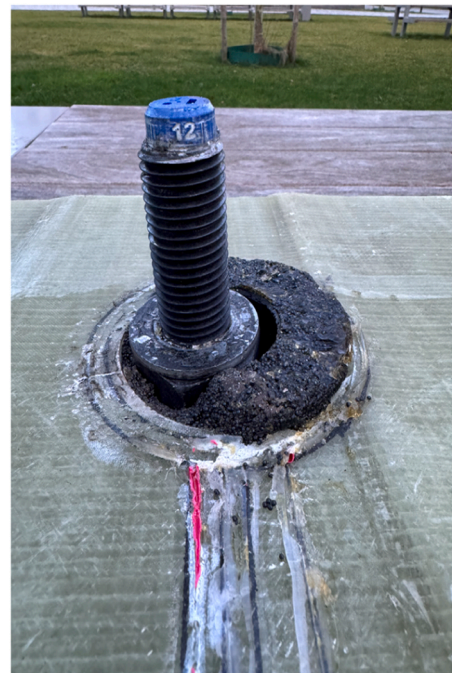
Fig. 9. Failure mode of re-tested iSRR connector subjected to fully reversed cyclic loading.
