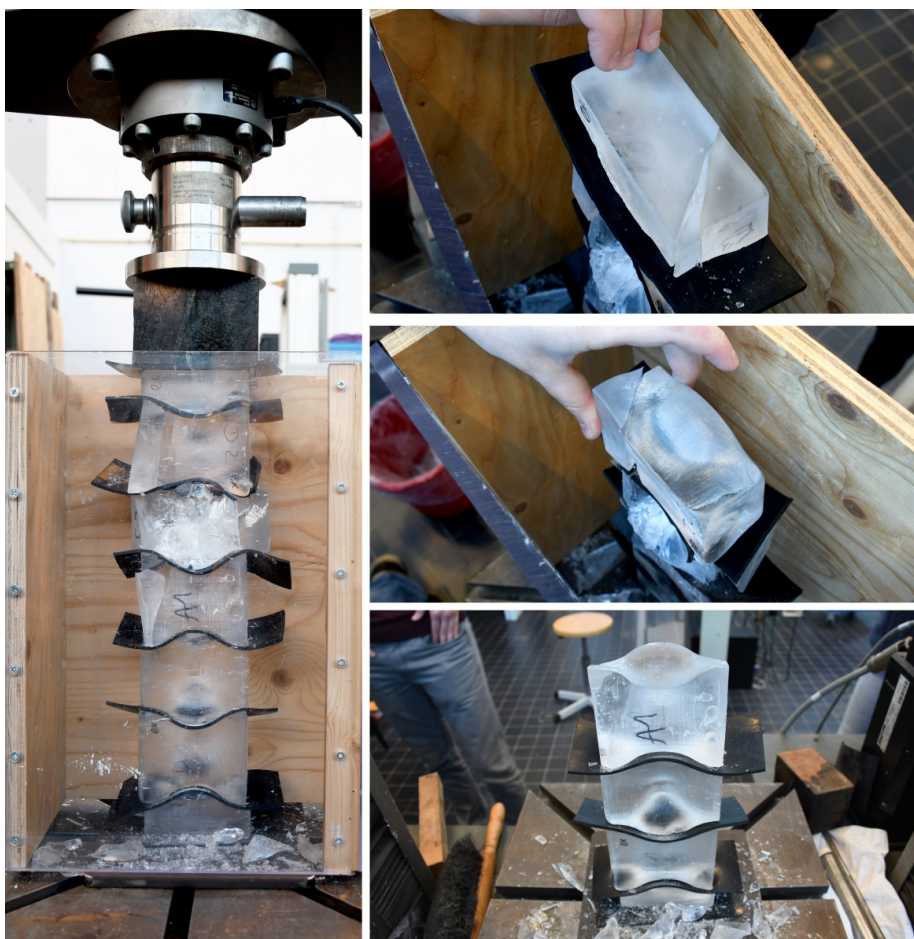
Figure 26: Specimen B after failure. Left: overview; Right: crack patterns in blocks a, b and d (top down). Block c was completely fragmented and could not be retrieved after the testing.
