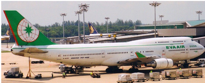
Figure 5.10: Example of an aircraft being loaded on ground with a tail support [95]
