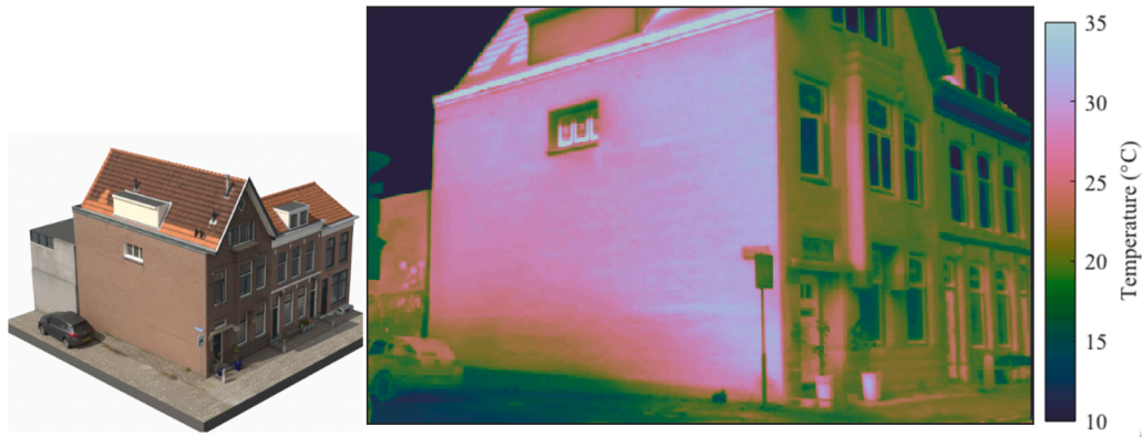
Fig. 2. Temperature on a façade from a thermographic image. The photograph shows a different temperature between neighbouring walls and a stark temperature decrease where the façade is in the shadow. Own images, see also [69].
